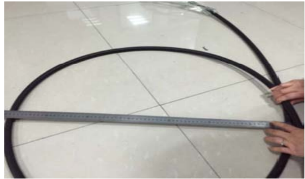
Figure 2a. Process of cable bending testing
