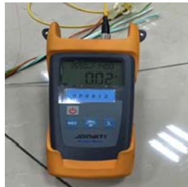
Fig 2b. The fiber attenuation after bending testing with 20D Bending radius
